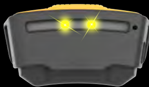
AutoSense Mode: 2 LEDs Flash Yellow When in Electromagnetic Field
